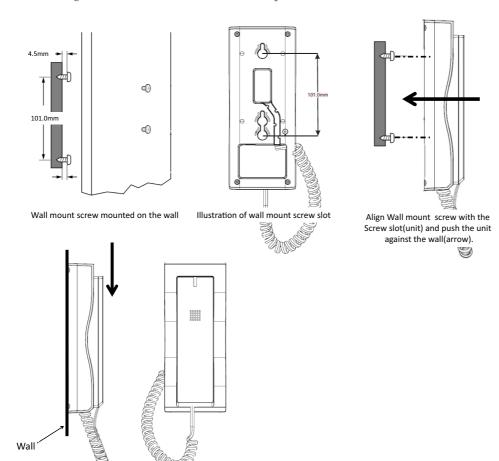
Slide unit downward(arrow) to lock unit to the wall.
